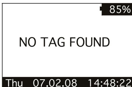
After a while the reading mode times out. The reader stops and shows the message "NO TAG FOUND".
