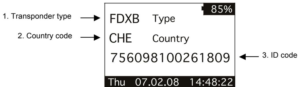
1. There are four main types of transponder: FDX-B and HDX are the ISO standard 11784/5. IDI stands for Destron, Avid, and PETRAC. The last type is TVN which stands for Trovan, AEG and similar transponders. When the reader displays the word "Industry" as transponder type, it means that this transponder is not coded for animals.
